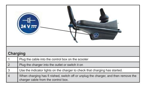
You are recommended to charge the batteries every night after you have used the scooter.
