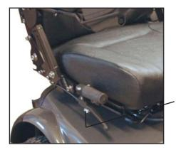
When using the handbrake as a parking brake, lock it in braking position by pressing the button in while applying the brake. To release the brake, press the button again.
