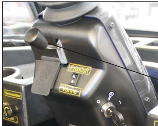
Adjusting the height of the handlebars.
