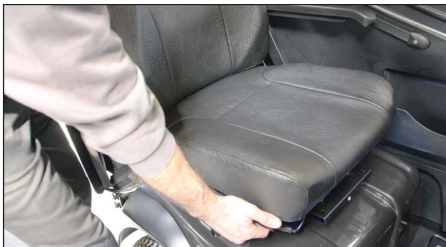
Lift the seat off the seat tube.
