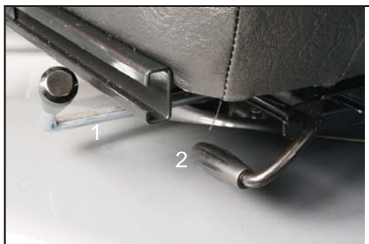
1. Release lever for seat rotation. 2. Release lever for seat forward/back.
