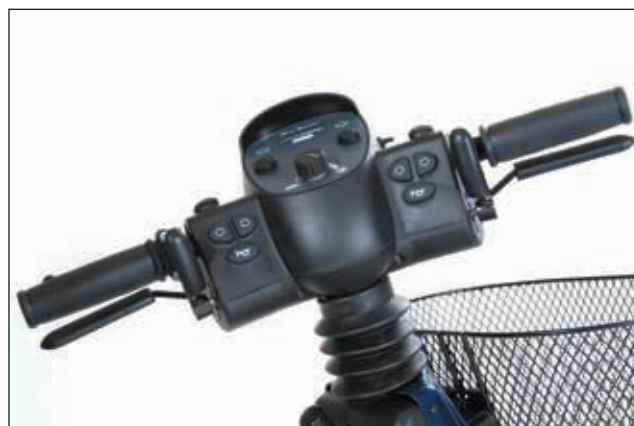
Left and right accelerator, with switch. M-127-06-171
