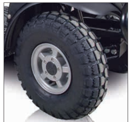
Wheel, complete 6". Ø370 mm, 530/4,50-6", black, 4 pr. for M-Model. T-127-3-765.
