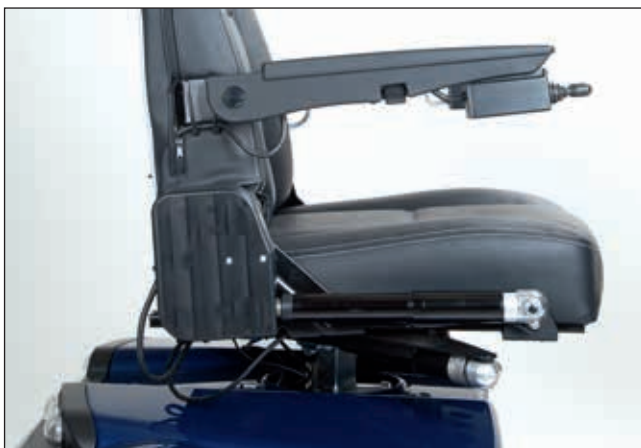
Seat can be moved up 15 cm. User weight up to 175 kg. M-127-07-159
