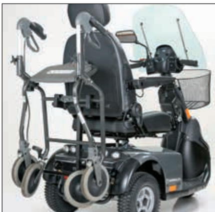
Walking frame carrier, max. weight 20kg (44lb). T-127-06-122.
