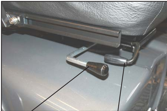
Release lever for seat rotation. Release lever for seat forward/back.
