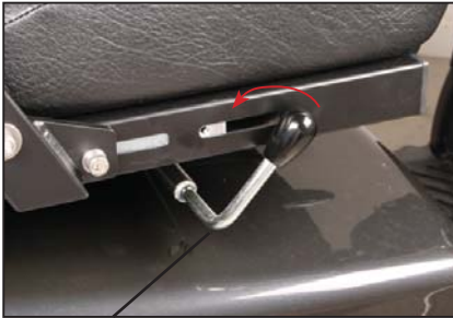
Release lever for seat rotation.
