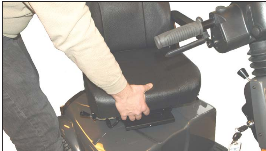
Lift the seat off the seat tube.
