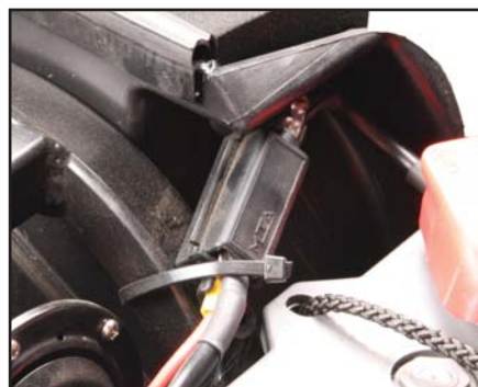
Main fuse 150 A. Located on each page under the battery cover, behind the batteries.
