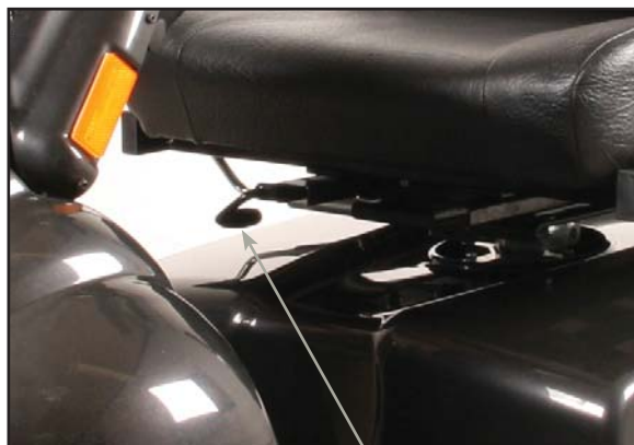
Release lever for seat forward/back.
