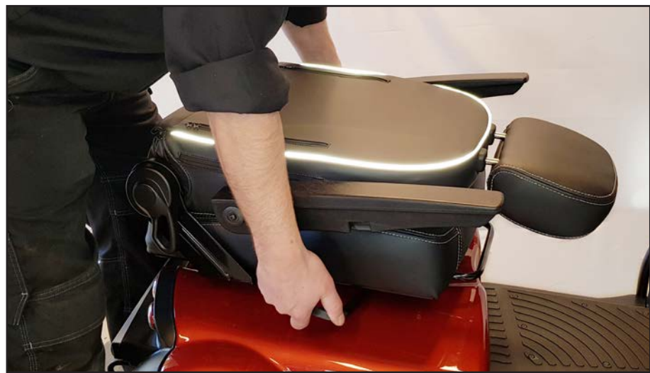
Lift the seat off the seat tube.
