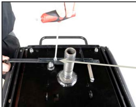
Out / in adjustment of the lever for rotating the seat
