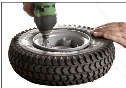
Remove the flange with the 5 screws (5 mm Allen key).
