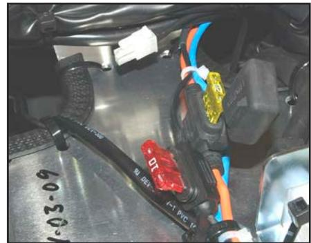
*Take the rear cover off. The plastic cover can be removed by squeezing the sides. Now the fuses can be replaced.*
