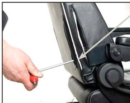
Unscrew the Allen screw and the armrest can be pushed up or down as needed. It can be adjusted 140 mm.
