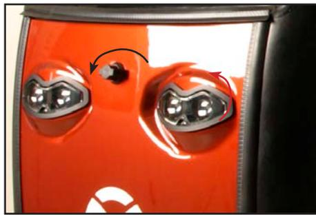
Open the front cover, by turning the handle 90° counter clockwise, and pull.
