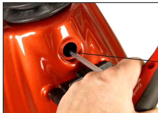
Adjusting the height of the handlebars.
