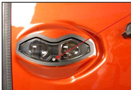
The headlight can be adjusted up/down by turning this screw.
