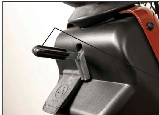
Adjusting the height of the handlebars.
