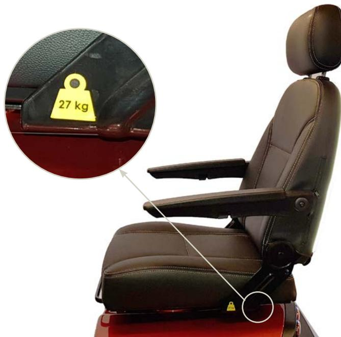
*This is our standard Ergo2 45 cm seat, the heaviest part of the X1 to remove. The label showing the seat's weight is located as shown above.*
