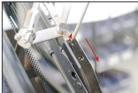
Lift carefully, so you can pull the wiper blade over the pin.
