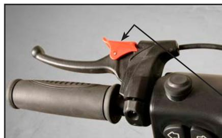
*When using the hand brake as a parking brake, lock it in braking position by pressing the button in while applying the brake.
