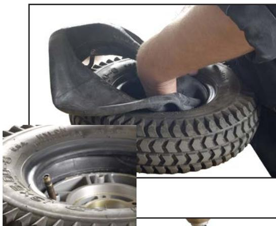
Replace or patch the tube. Ensure that there are no foreign objects in the tyre before the tube is replaced. Pump air into the tube so that it is positioned correctly in the tyre, but do not fill it up completely yet.
