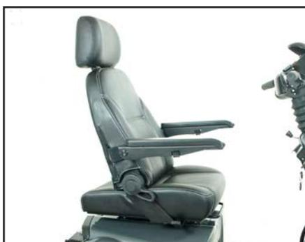
The depth of the seat can now be adjusted by sliding the seatback forward and back.
