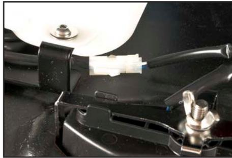
Remove the headlight. Detach the plug, and it is free to change.
