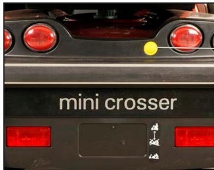
*Electronic disengagement. Works only when the scooter is turned on.*
