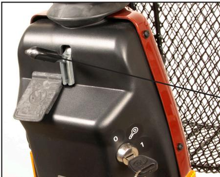
Adjusting the height of the handlebars.
