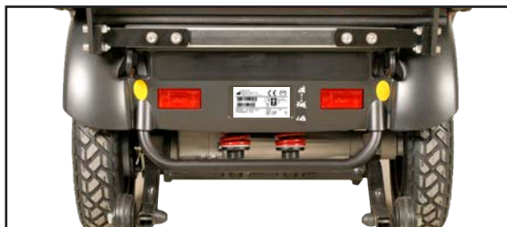
Position of serial number plate on vehicle.
