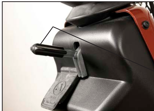
Adjusting the height of the handlebars.
