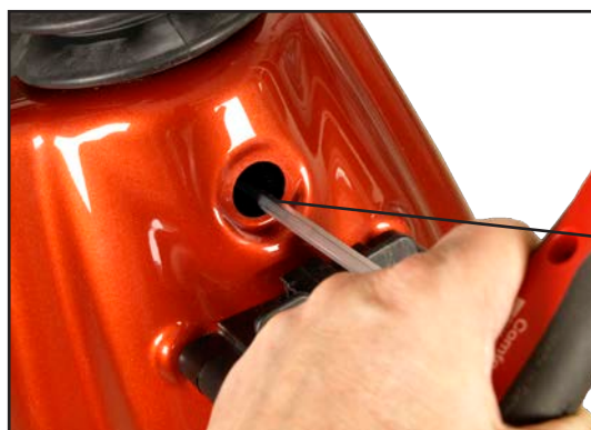
Adjusting the height of the handlebars.
