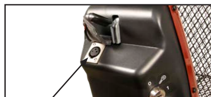
Connect the charging plug to the 3-pin socket on the steering column. The charging socket is located under the protective cover.
