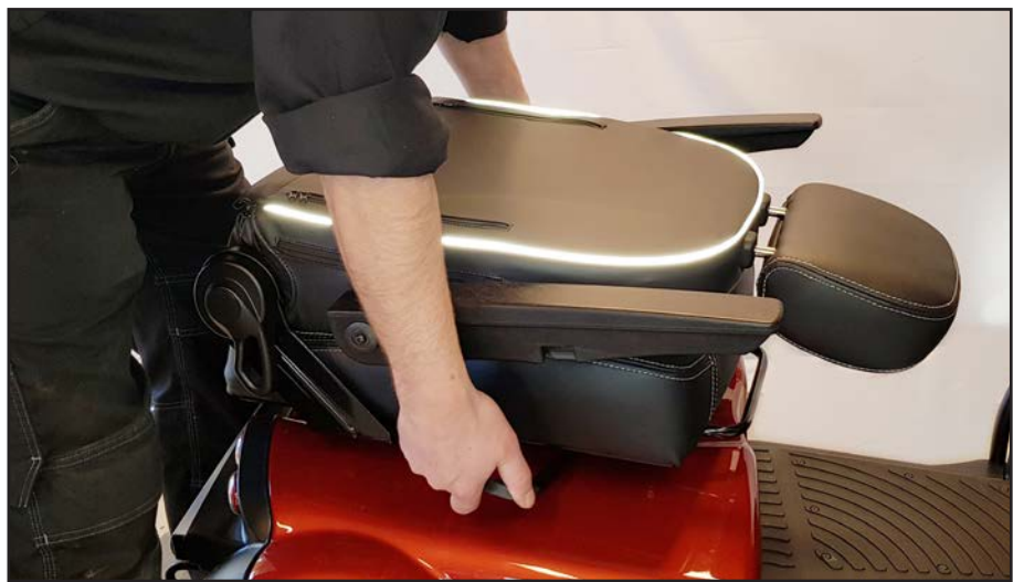
Lift the seat off the seat tube.
