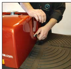
Remove the thumbscrew and remove the battery cover.
