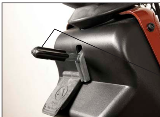
Adjusting the height of the handlebars.
