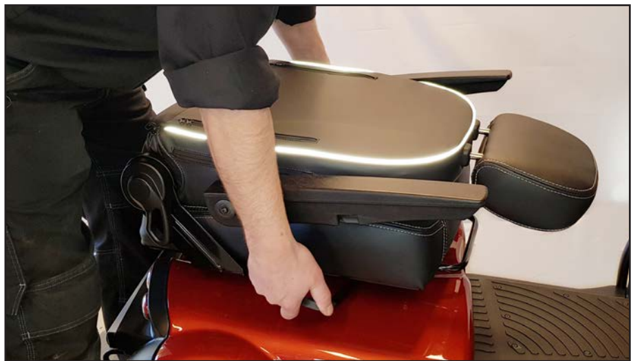
Lift the seat off the seat tube.
