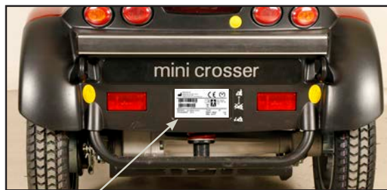
Position of serial number plate on vehicle.
