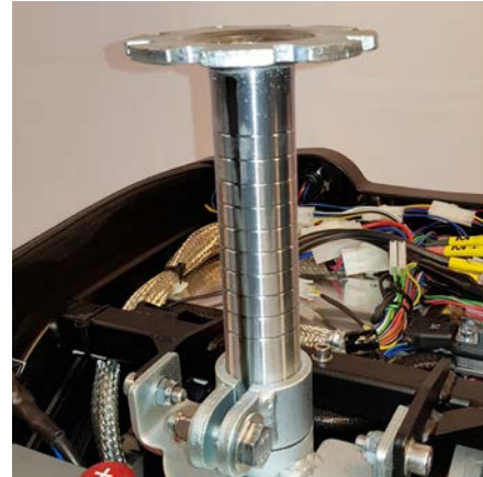
Adjust the seat post to the desired position. The seat post is marked with a ring at each centimetre.
